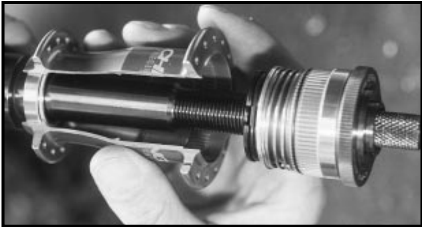
Figure 23 - remove RingDrive™ assembly
