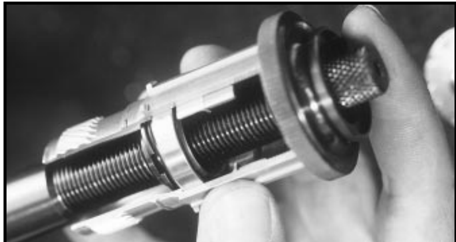
Figure 24 - remove drive shell bearing
