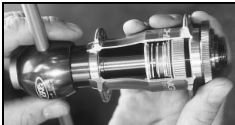
Figure 33 - press drive side bearing
