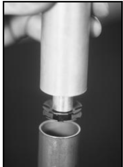
Figure 3 - starnut installation tool
