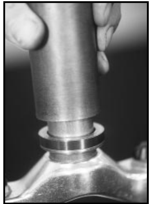
Figure 2 - setting the baseplate
