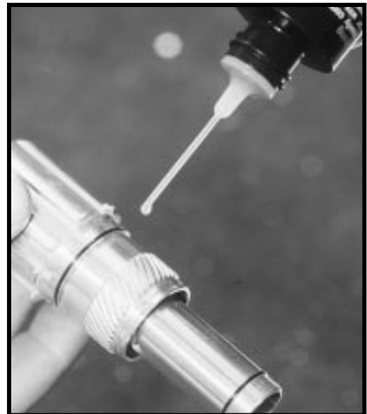
Figure 14 - lube helical splines
