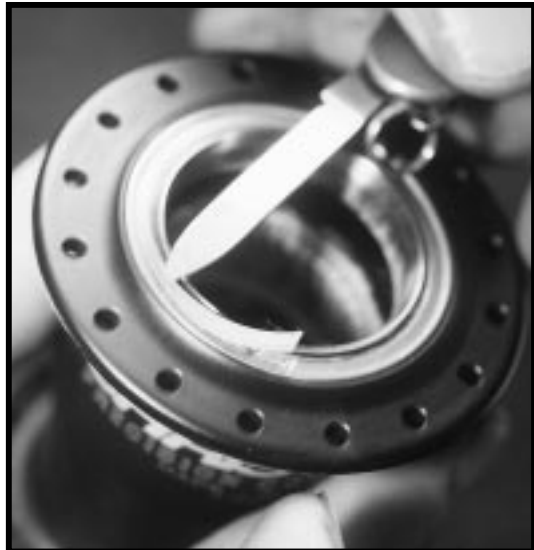
Figure 12 - remove snap ring
