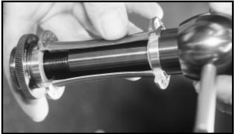
Figure 19 - press front hub shell bearings
