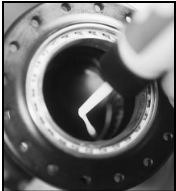
Figure 13 - lube RingDrive™ teeth
