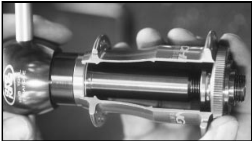
Figure 27 - install non-drive side bearing
