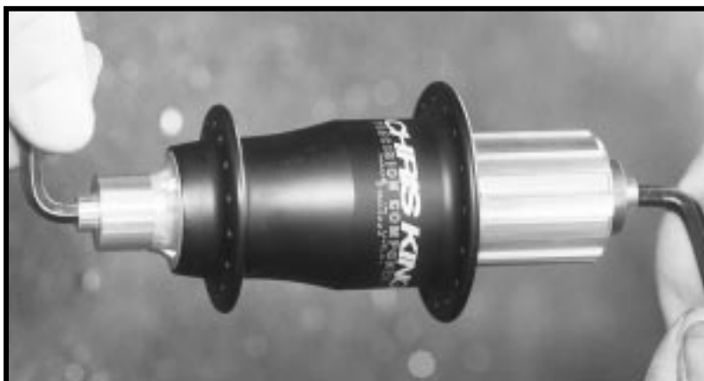
Figure 11 - disassemble main axle
