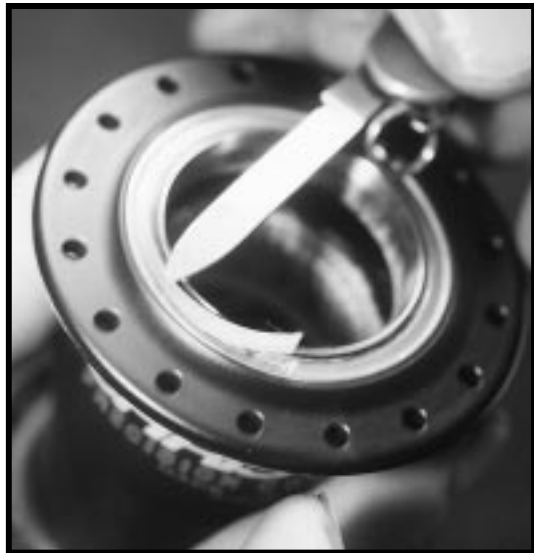
Figure 26 - remove snap ring
